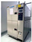
Environmental test chamber Hot and cold impact testing machine
