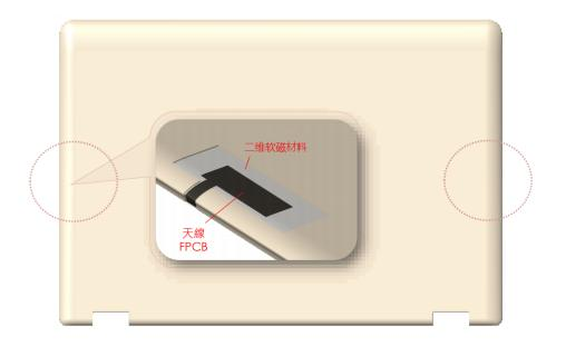
In this application, the two-dimensional soft magnetic material shielding the impact of the backplane on the antenna is a key component to improve the communication efficiency of the antenna.
