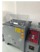
Salt spray test chamber
